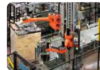
6 END-OF-LINE The final stage of packaging, including palletizing and wrapping, guaranteeing product protection, load stability, and smooth logistics downstream.
