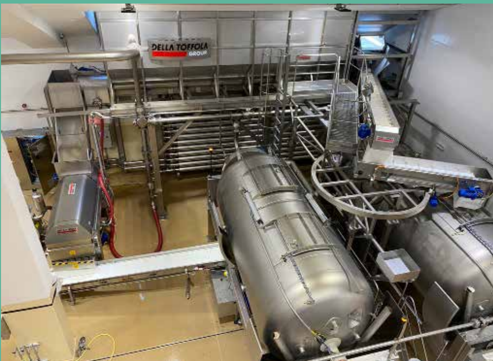
On the right: process of receiving grapes and pressing in an inert atmosphere
